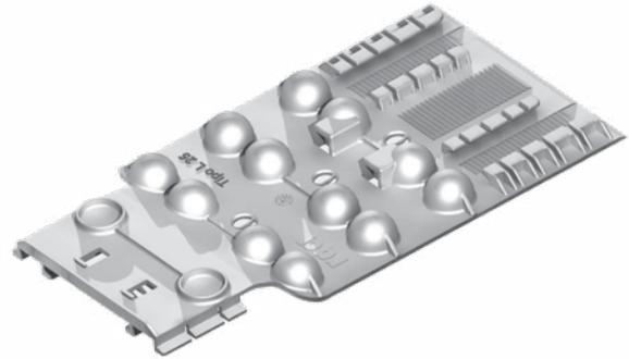
Each spacer element represents a flexible section that has a toothed male butt strap at one end and an appropriately toothed female slot on the other end. Absolutely no metallic parts are involved in their assembly. This design allows for on site adjustments for any variances within the O.D. range. Coupled with their flexibility they cover all types of pipe from O.D. range 1.65 inches (42 mm) and upward.
